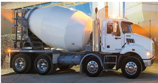
Figure 9.2 – Transit Mixer (aka concrete Agitator or ‘Agi’)
