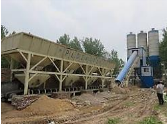
Figure 9.3 – Continuous Mixer (aka 'Pug Mill')
